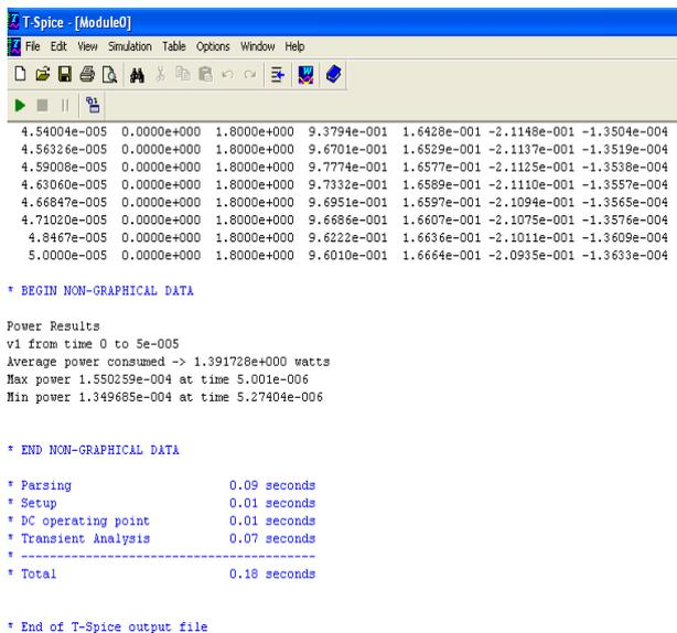
Fig. 7. Power analysis of current conveyer based sense amplifier
