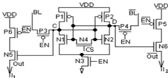
Fig. 3. Bit-line decoupled latch
