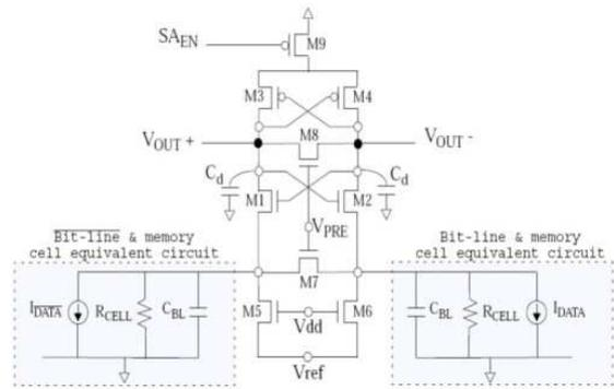
Fig. 5. Clamped Bit Line Sense Amplifier
