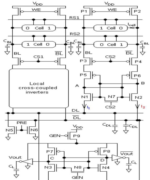
Fig. 4. Proposed design coupled with a simplified read-cycle-only memory system
