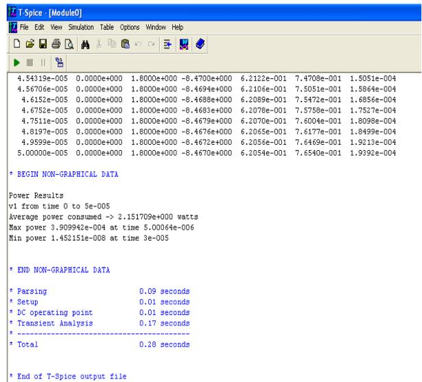
Fig. 9. Power analysis of alpha latch
