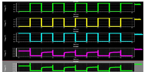
Fig. 10. Waveform for bit line decoupled latch sense amplifier
